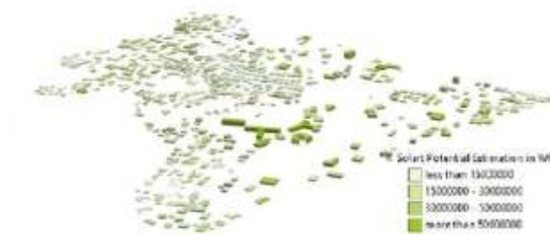
**Figure 15: Rooftop Solar Potential Estimation in Wh**
